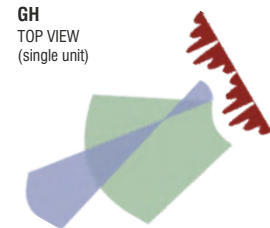
G - VERTICAL DIFFUSION WITH COMPRESSION EFFECT. H - VERTICAL DIFFUSION WITH SCATTERING EFFECT.
