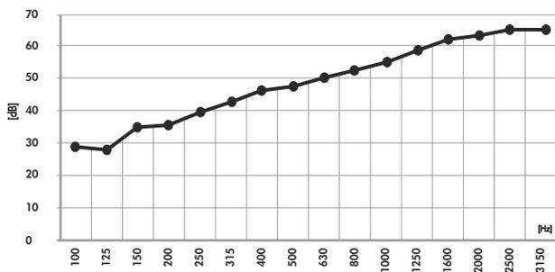
● 13mm plaster + 110mm ceramic brick + 13mm plaster+ ECOiso® SPL® 60mm
