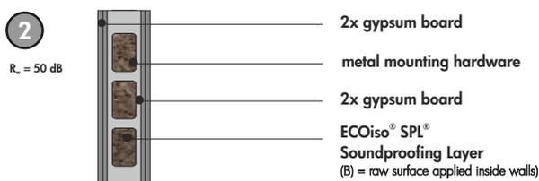
2x13mm gypsum board + ECOiso® SPL® 60mm on metal frame + 2x13mm gypsum board
