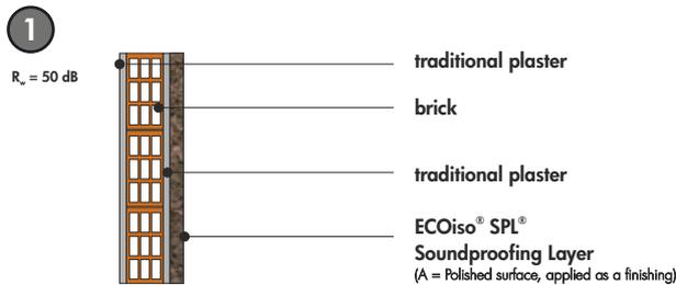
13mm plaster + 110mm ceramic brick + 13mm plaster + ECOiso® SPL® 60mm
