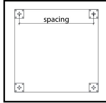
Locate the metal brackets on the back of the panel and measure and take note of each "spacing".
