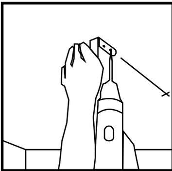
Use a screwdriver to attach the 4 mounting L-shaped metallic accessories to the ceiling. Fit the panel between the L-shaped metallic accessories and screw them to the sides of the panel.
