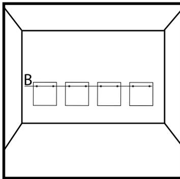
With a level define the "B" line, then mark on it the measured spacing, and two suspension points per panel on the wall. After verifying all measurements, drill 2 holes on the wall per panel, install both sleeves and 2 screws. Leave the tip of the screws approx. 5 mm from the wall.
