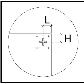
Measure "L" and "H" distance on the back of the panels on both sides.
