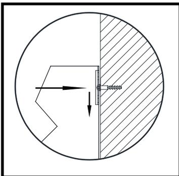
Slide the panel so the center back cavity on the metal plate enter the 2 screws and gently slide it down.
