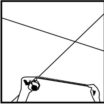
To determine the placement of the panel use a marker, a measuring tape and a ruler to mark the needed 4 points per panel on the ceiling. Placement aprox. 15cm from the vertices of the panel. Make 4 drilling points on the ceiling and insert the sleeves in the ceiling.
