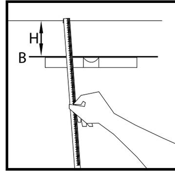
Measure the placement of the panel using a tape measure, a pencil, a ruler and a level. From the top panel line, measure and orthogonally mark the "H" distance.
